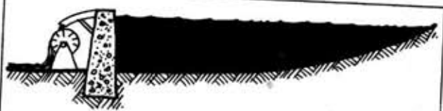
FIGURE 7.13 CHECK DAM FOR RAM PUMP OR WATER WHEEL Only 1-3 m of head enables modest energy use for mechanical power, lift pumps, or diversion to canals.
