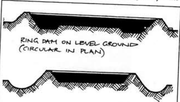
FIGURE 7.9 RING AND TURKEY'S NEST DAM. Hold water pumped in by a windmill and provides a low head in flat landscapes; can be pipe-filled from a large roof or from parking areas.
